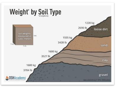
mixtures of the different types of soil (sand, clay, silt and rock) necessitate different safe slopes from one excavation site to the next.
